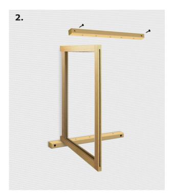
Using one of the panels as a guide, measure the approximate height & position that the top piece of the base must be installed.
