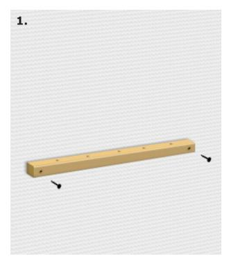
First decide on the height you would like the finished browser to be, then mark the positions of the holes on the bottom base piece.
