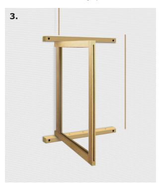
With the 2 base pieces installed, place one of the panels between them, and align it with the base pieces holes.
