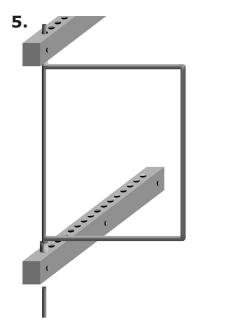
Place the frame inside the base and align it with the holes. Then simply push the pin up through the bottom of the base and tighten the screws
