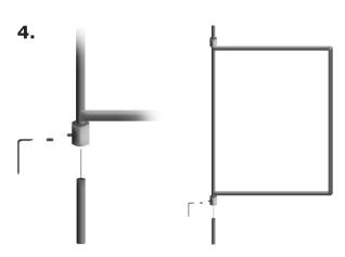
Remove the bottom pin from the sleeve frames by un-screwing the bolts on the lower end of the cylinder.
